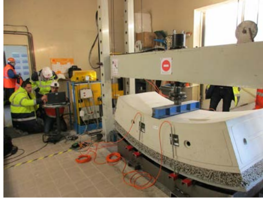
Figure 8: First tests carried out to check VMC resistance to handling
