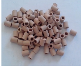
Figure 5: Ceramic shells produced from argillites (i.e. from raw material excavated in the Bure URL)
