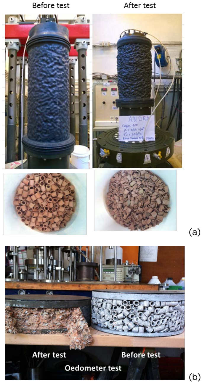
Figure 7: Geotechnical test (a) triaxial test on ceramic shells, (b) oedometer tests carried out with the ceramic shells and concrete
