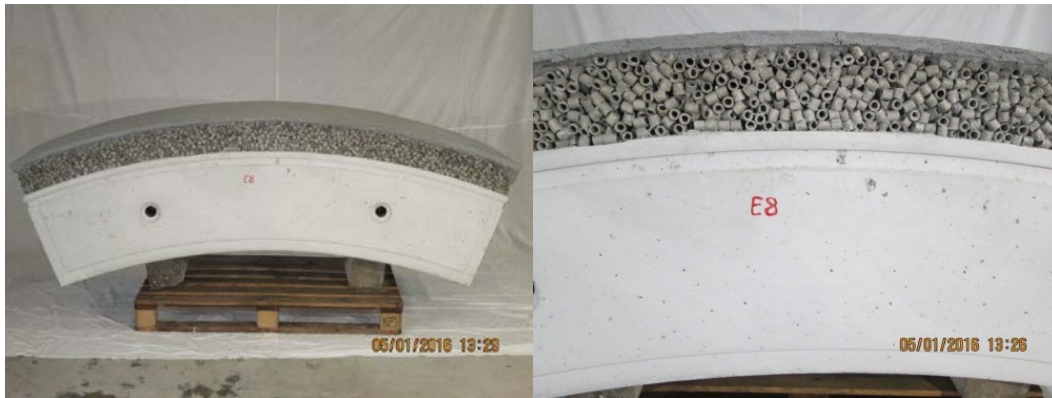
Figure 4: VMC prototype (left) and its compressible material coating (right) for GVA test drift
